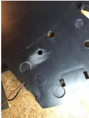
Roughen the surface of the base (underside, of course!) next to the 5mm hole using a fine file or emery paper.
