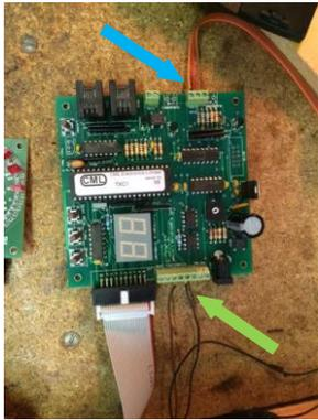
This photograph shows the turntable wiring to the TXC1.
