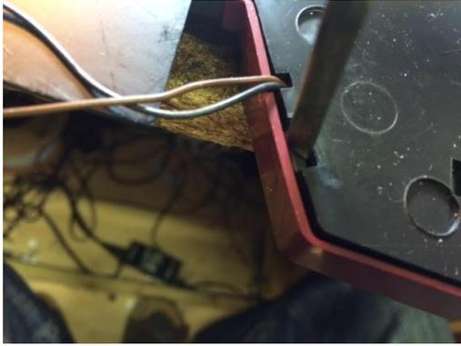
Insert a screwdriver as shown. Carefully twist and then move outwards to ease the side of the plinth away from the base (by a few mm only – do not use excessive force!).
