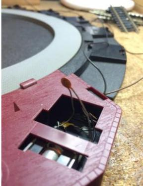
This is the position of the capacitor which allows the plinth to be removed from the base.
