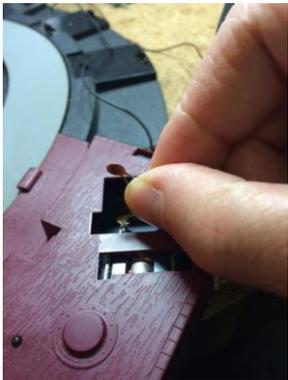
Bend up the leads on the motor suppression capacitor so that the capacitor is clear of the plinth.
