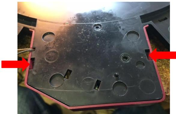
Turn the turntable over, and identify the apertures for the plinth retaining clips.
